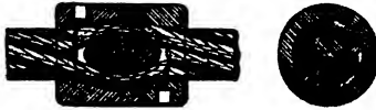
FIGS. 33 and 34.—Modified Form of Otto Knot or Carrier Collar. Longitudinal and Cross Sections.
